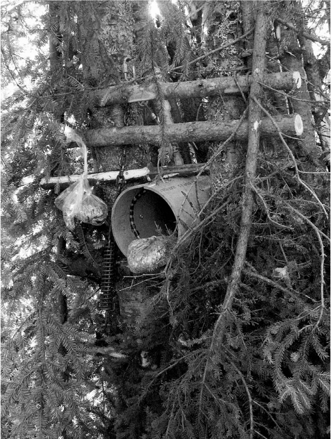
Fig. 6. Completed installation of the RL04 trap. Dense vegetation placed around the trap and additional bait bags placed near the trap opening directed bears to the front of the trap.
