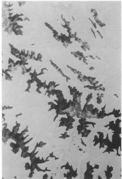
Fig. 5 Scene 1 with high-altitude overlay superimposed in white light. Only the areas above 2100 m remain visible.
